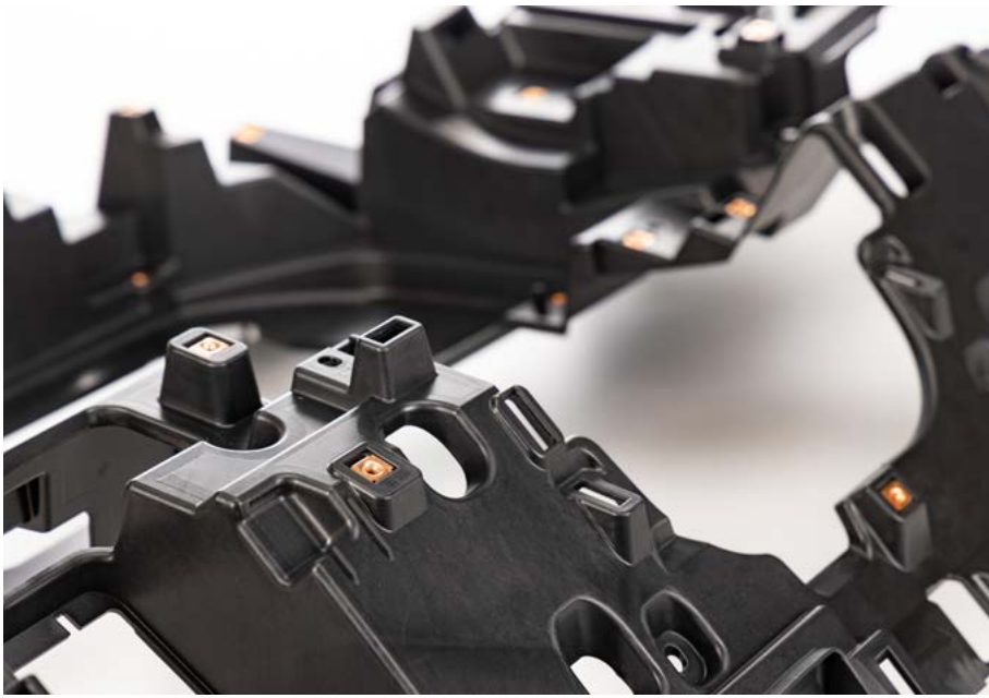
All 16 grades of Geon's Resilience R PP come in black or grey and are UL94 HB approved. In addition to glass and glass/mineral reinforcement, there are several mineral-filled formulations containing either talc, mica, calcium carbonate or barium sulfate, as well as a neat grade. Potential applications include instrument panel carriers like that shown here. Courtesy of Geon Performance Solutions
